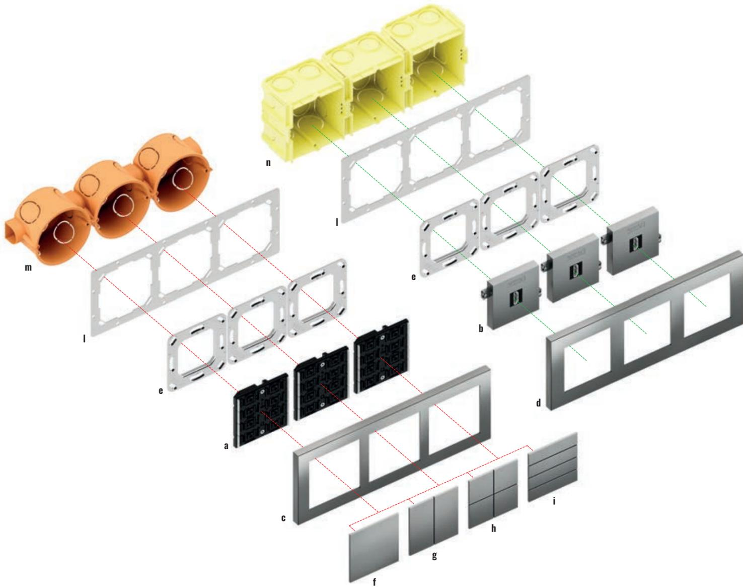
Keystone modules compatible with Ekinex civil series. Wide range of devices to integrate network systems, multimedia systems and antenna systems. The front covers can be declined in the various colours available, thanks to a special painting process that allows them to be chromatically matched to the other wall devices.
