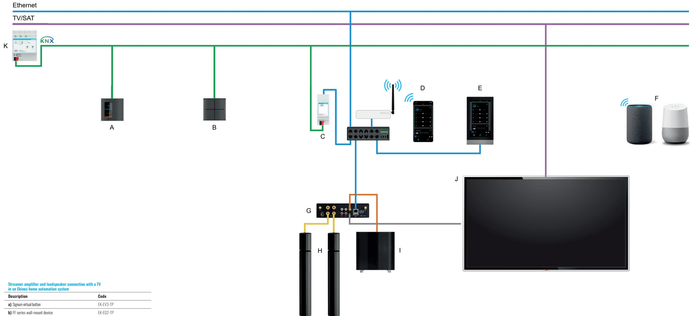
**Streamer amplifier and loudspeaker connection with a TV in an Ekinex home automation system**
