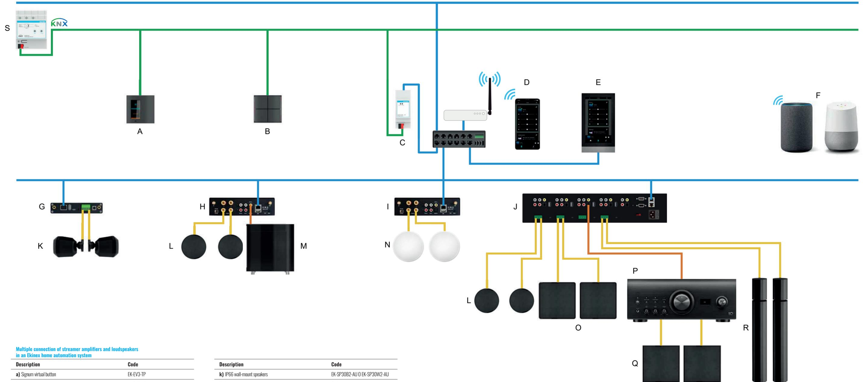
Multiple connection of streamer amplifiers and loudspeakers in an Ekinex home automation system
