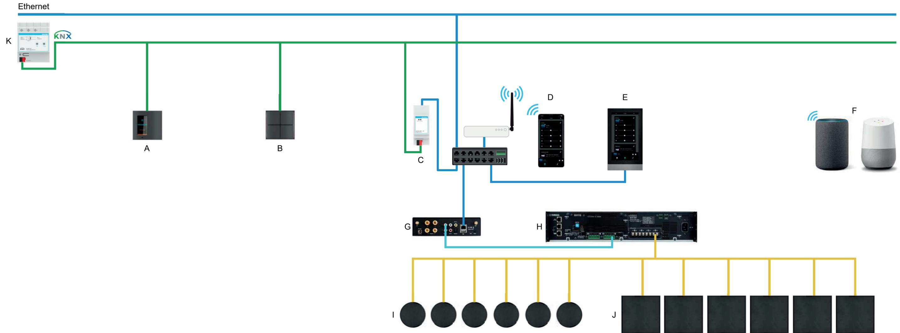
**Streamer amplifier and speaker connection with an external 100V amplifier in an Ekinex home automation system**
