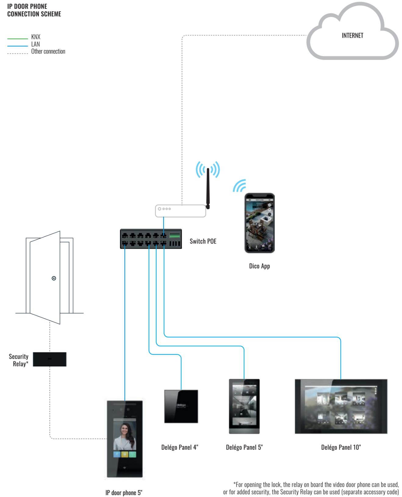
\*For opening the lock, the relay on board the video door phone can be used, or for added security, the Security Relay can be used (separate accessory code)
