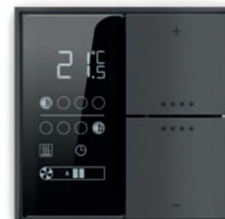
The thermostats simply get connected to the unique signal bus cable and do not require auxiliary power supply; the devices are powered at SELV (Safety Extra Low Voltage) voltage, thus offering a much higher safety level than traditional commands. The configuration and commissioning is carried out by means of the ETS® software. The related application programs can be downloaded from the [www.ekinex.com](http://www.ekinex.com) website.
