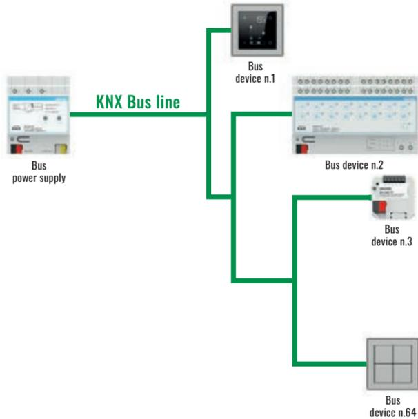
It is necessary to respect KNX topology prescriptions while designing the system, in order to guarantee communication within the system:
